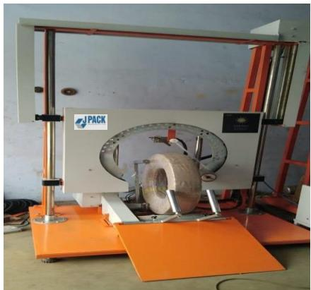
The machine is designed for Cable Coils, Tyres, Irrigation coils, Pallet Wrap machine, Box stretch rapping machine, Garden pipe wrapping machine. Coil wrapping machine need stretch film roll is stretched to the required Percentage and wrapped around the Product in inside out direction by using a Stretch Wrapping machine..
